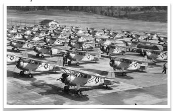
In 1942, the GH-2 "Nightingale" model was introduced as an aerial ambulance for the US Navy of which 131 were built. And, in 1943, 115 GH-3's (a variant of the GH-1 with equipment changes and a 122-gal fuel tank) were built as personnel transports. GH-3 USN BuNo's: 44921/44922, 44935/44937, 44939, 44941/45049.
