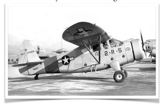
as the GH-1 model which was a communications and liaison version of the DGA-15P, built for the United States Navy and United States Coast Guard; consisting of 29 which were built new and four impressed civil aircraft.
